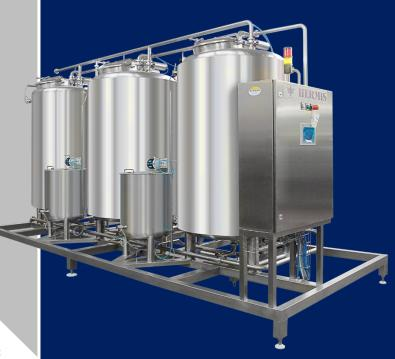
CIP station is designed for sanitary cleaning of pipelines, buffer tanks, bottling lines, pasteurization plants to remove contaminants without the need of equipment disassembly.
