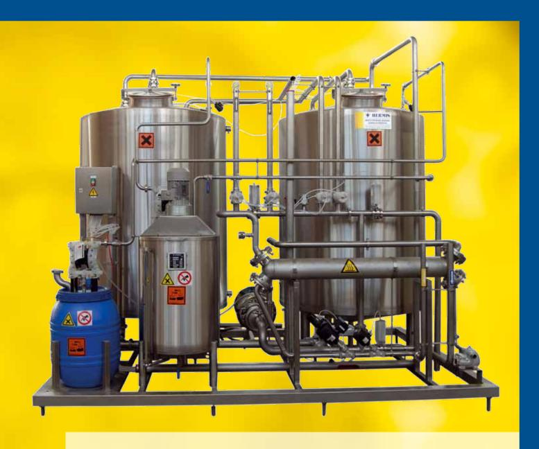
Automatic station CIP is designated for in-place sanitation and washing of pasteurizers' heat exchangers and pipes, filling blocks and buffer vessels.
