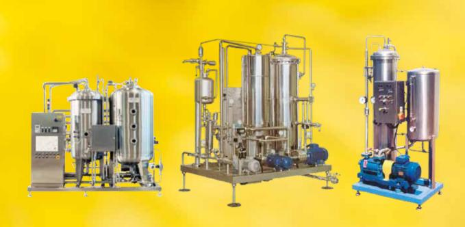
**Mixer saturator** is designated for production of sweet carbonated drinks and carbonated mineral water. The machine consists of high-precision equipment and is operating in automatic regime for easy mixing and carbonization. This machine may be used for carbonization only.
